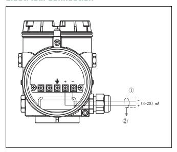
Electronics and terminal compartment, double chamber housing
